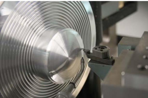
Fig. 4 Machining freeform surface on the lathe(Freeform700A).
