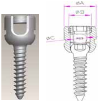
Fig. 1 Three Design Factors(A · B · C) of Locking System in Poly-axial Pedicle Screw
