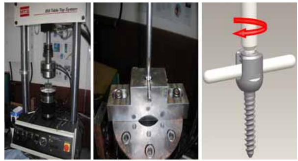
Fig. 2 Torque Tests by MTS System
