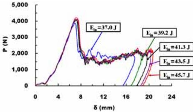
Fig. 3 (a) Results of impact analyses of SUS304H panel (P-δ curves)
