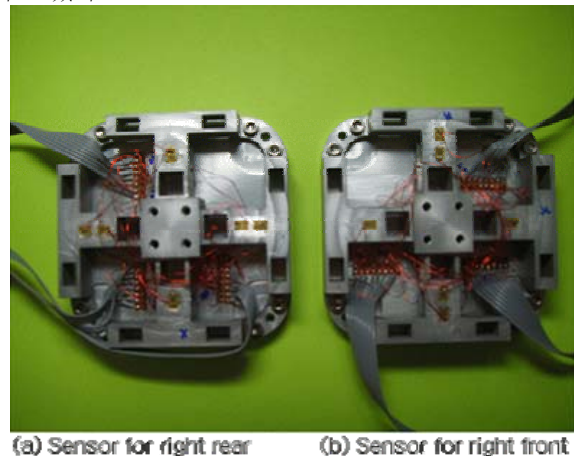
(a) Sensor for right rear (b) Sensor for right front Fig. 2 Photograph of the developed two 6-axis force/moment sensor for intelligent right shoe
