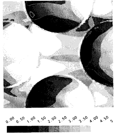
Fig. 3 Nusselt number contours for optimum shape ( \beta=0.09 )
