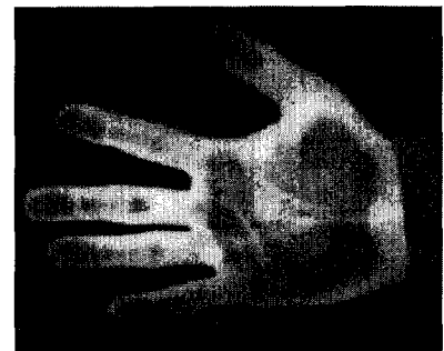
Fig. 1. The infrared image of a 300K object (human's hand) captured with the DWELL QDIP at 60 K.
