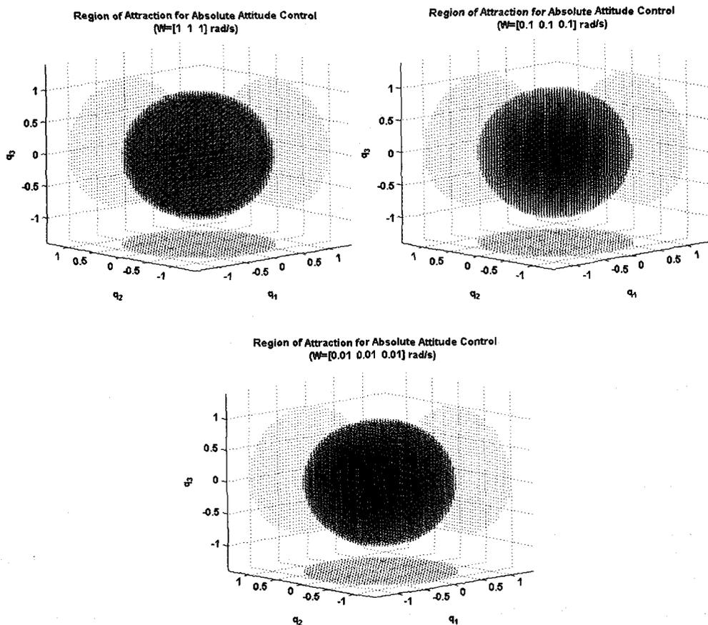
Figure 1. Region of attraction for absolute attitude control system under different angular velocities.
