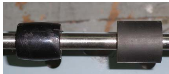
Fig. 5 Crown pulley and flat pulley
