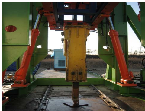
Fig. 3 Break noise measurement system
