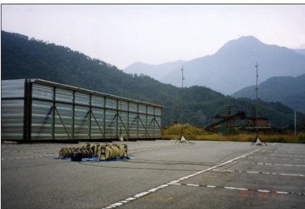
Fig.1 The conventional estimation method of the noise barrier's acoustic performance using in Japan.
