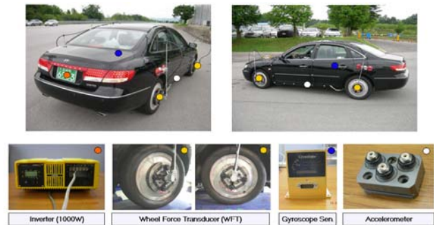
Fig. 1 Measurement sensor and position
