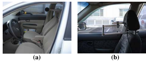
Fig. 3 The set up point of the sound level meter(a) and microphone(b)
