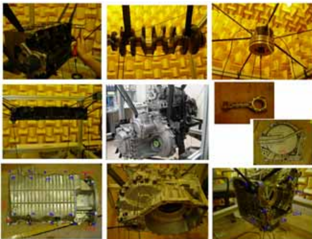
Fig.3 Modal testing of powertrain system
