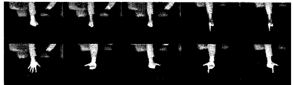
Fig. 6. The hand gestures. 1st col : Power On/Off, 2nd col : Channel Up, 3rd col : Channel Down, 4th col : Volume Up, 5th col : Volume Down
