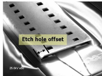
Fig. 2. Fabricated filter and definition of etch hole offset
