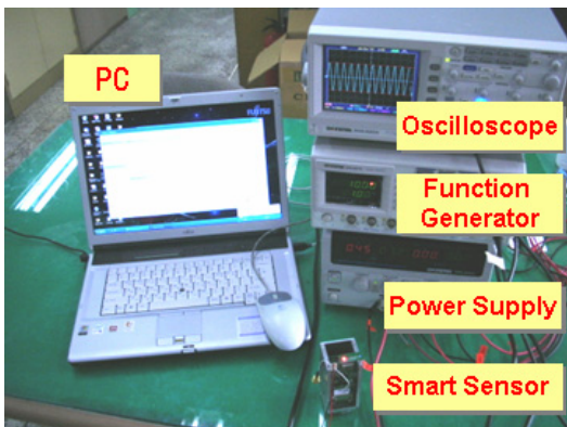
Fig. 10 Test setup for test of analog and digital signals
