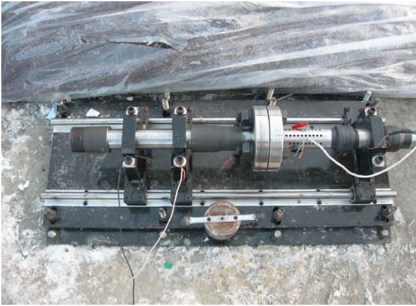
Fig. 4 Launcher & Muzzle Breaker Tube of the soft recovery system
