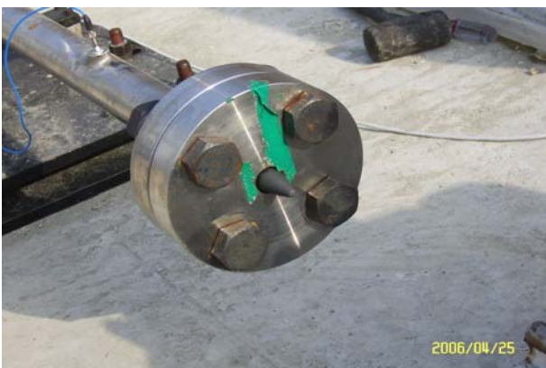
Fig. 6 A Vulcan ball stop at end of pipe in the soft recovery system
