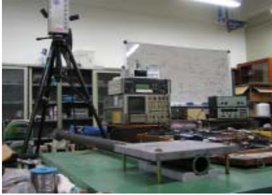
Fig. 1 Experimental setup for measurement of vibration signals of a gun barrel type structure
