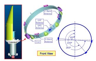
Figure 1. Placement of the GPS Antennas on KSLV-I.
