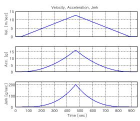
Figure 5. Velocity, Acceleration and Jerk in the Scenario.
