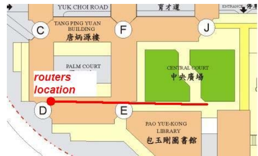
Figure 6. Test site at the Podium level of the Hong Kong Polytechnic University for the determination of the relationship between the signal strength and the distance
