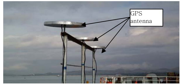
Fig 9 GPS/MIMU attitude determination system set-up on the ship
