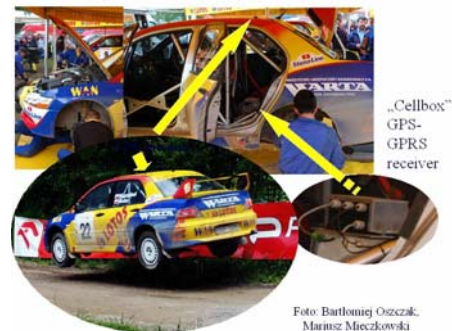
Figure 12. Localisation of GPS components on the cars.
