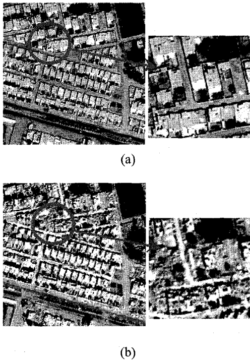
Figure 2 Subset of Quickbird images (a) undamaged areas (b) damaged areas: (Images: curtsey of CSR, University of Texas.)
