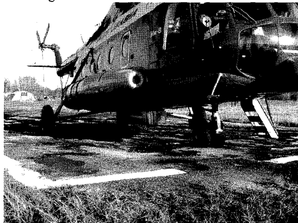
Fig. 1. MI-8 helicopter with antenna radome installed underneath before flight.
