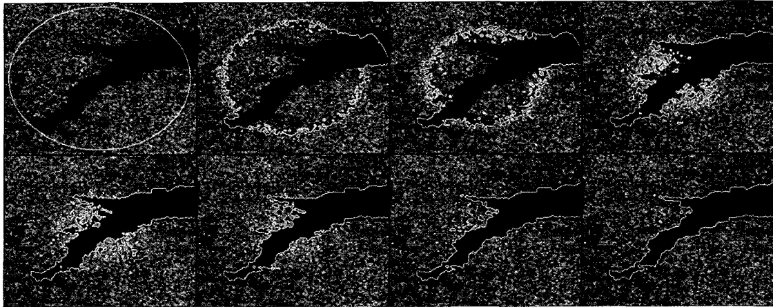
Figure 3. Different steps of the curve evolution model starting from an initial arbitrary elliptical curve and the final oil spill detected boundaries. View the figure starting each row from the right.
