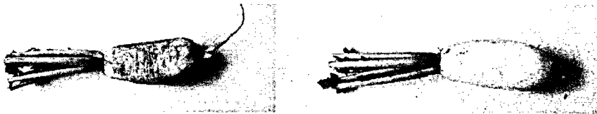
Fig. 5 Radishes before and after processed on the blade belt type peeling device.
