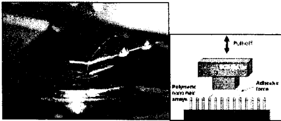
Fig. 7 Diamond-shaped cantilever in AFM system for adhesive test
