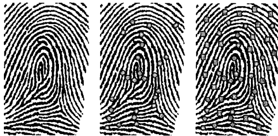
Fig. 2. Example of Generating Protected Templates[19]; (a) Example of a Fingerprint, (b) Example of a Typical Template(circles: real minutiae extracted from (a)), (c) Example of a Protected Template(circles: real minutiae, rectangles: chaff minutiae).
