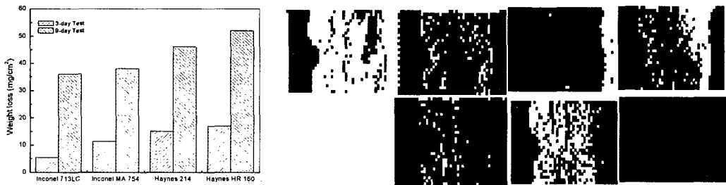
Fig. 1. Corrosion rate of tested alloys. Fig. 2. Cross-sectional SEM image and elemental distribution of Inconel 713LC.
