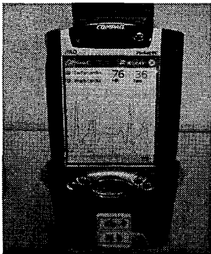
Figure 5: A real-time normal ECG monitoring at PDA
