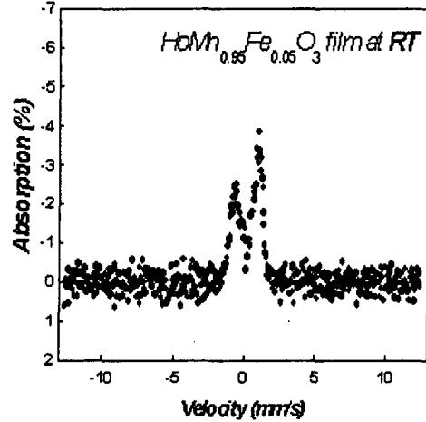
Fig. 2. Mössbauer spectrum of  $\text{HoMn}_{0.95}\text{Fe}_{0.05}\text{O}_3$  thin film.
