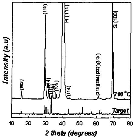
Fig. 1. XRD patterns for  $\text{HoMn}_{0.95}\text{Fe}_{0.05}\text{O}_3$  target and thin film.
