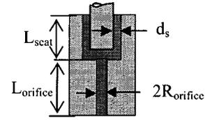
Fig. 9 Orifice of nozzle and valve cap
