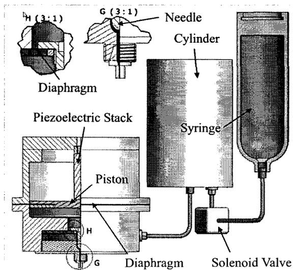
Fig. 1 Schematic diagram of the hybrid dispensing system
