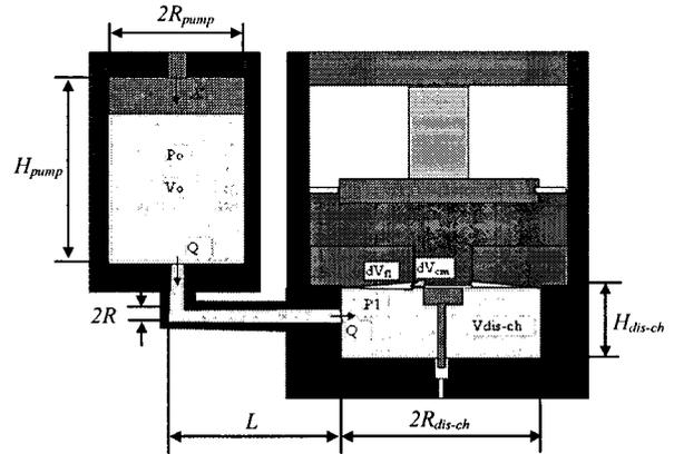
Fig. 10 Schematic diagram of fluid dynamic model
