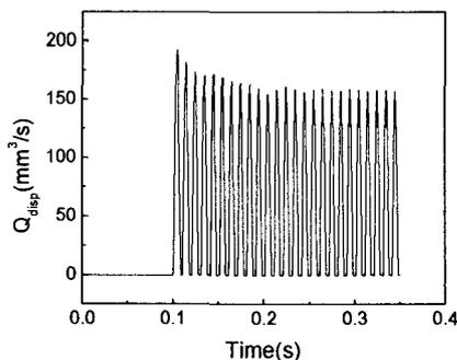
Fig. 11 Dispensing flow rate
