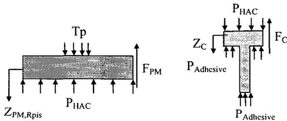
Fig. 6 Schematic diagram of piston and needle
