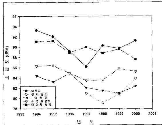
Fig.2 Trend of Automobile Noise Level for Exhaust System
