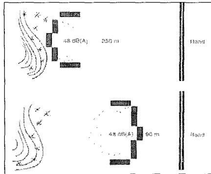
Fig. 3. Noise Reduction Effect along with building arrangement
