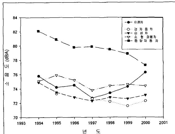
Fig.1 Trend of Automobile Noise Level for Acceleration System
