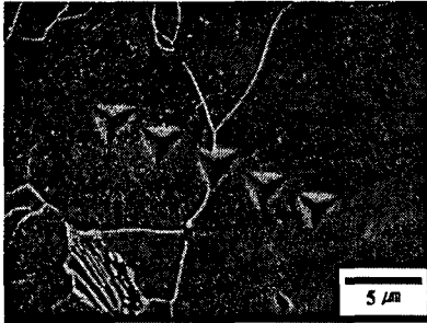
Fig. 5 SEM micrographs of indentation, Effect of grain boundary in ferrite
