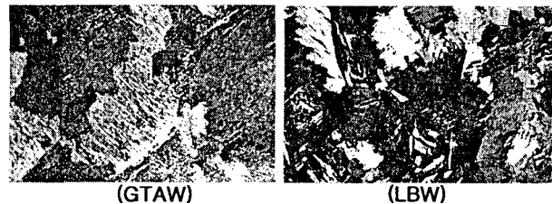
Fig. 6 Microstructure of weld metal of GTAW and LBW (250:1)
