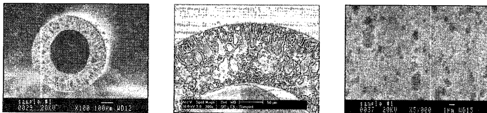
Fig. 1. SEM images of prepared PES hollow fiber membranes.
