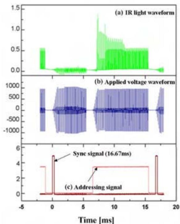
**Figure 5: Operating waveforms and driving signal Infra Red light waveform (a), proposed driving waveform (b) and gate signal for addressing(c).**
