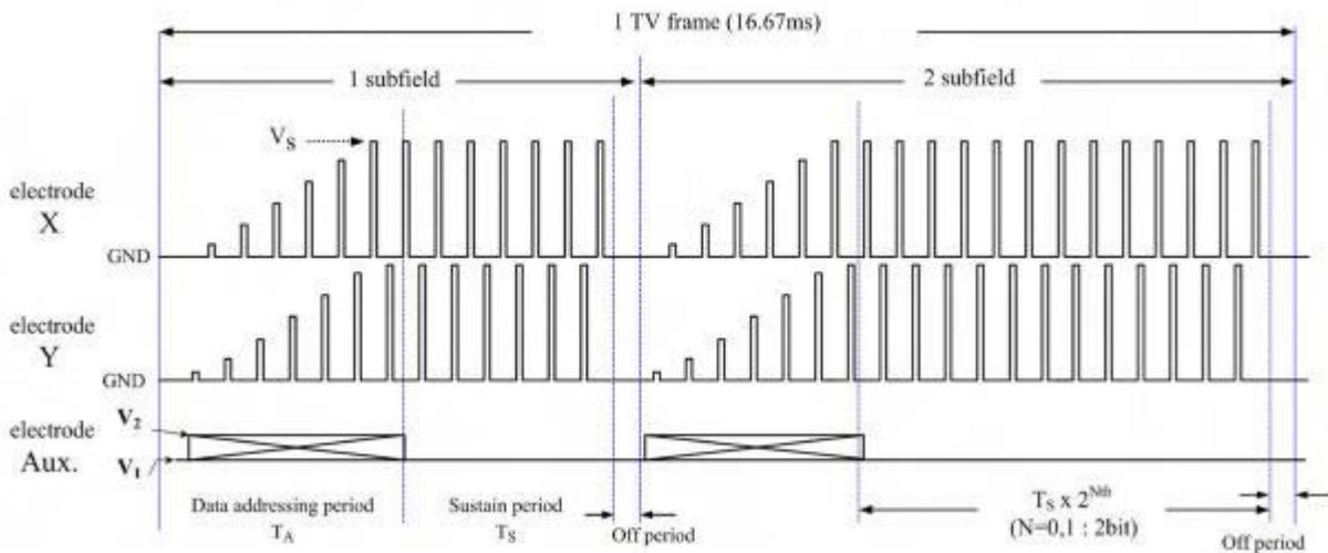
Figure 4: Drive waveforms for the areal selective 2-bit dimming
