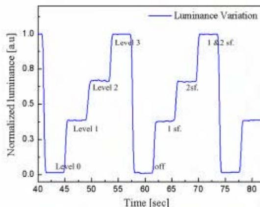
**Figure 6: Luminance variation on the proposed sub-field driving method**
