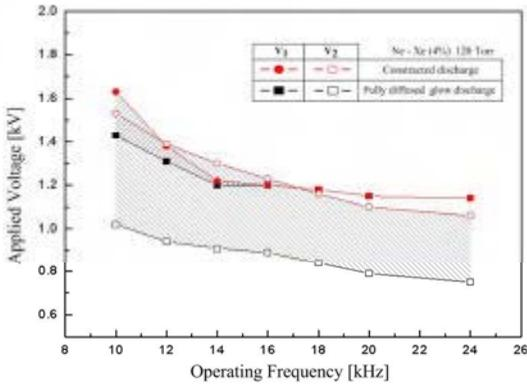
Figure 2: Operating voltage margin
