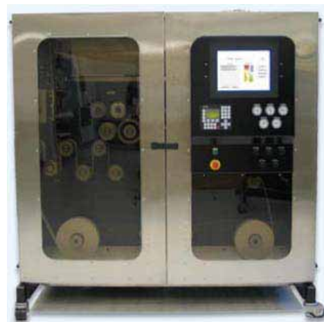
Figure 3. Roll-to-roll ink jet printing equipment by iTi Corporation. [2]
