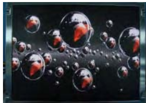
Figure 7 Photograph was taken from a 20.1" S-IPS that was fabricated using the manufacture technology with PI film after IBA process.
