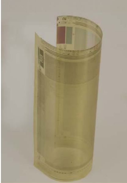
Figure 2. 50 x 50 mm a-Si TFT array on 3 µm thick freestanding polyimide layer made by the EPLaR process.
