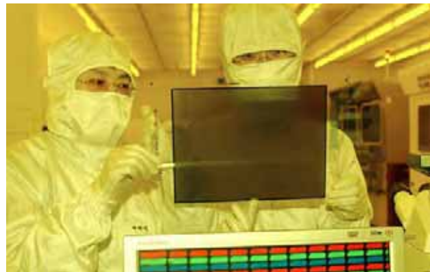
Figure 4. 14.1" LCD color filter by inkjet printing technology in 2005.
