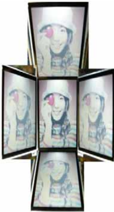
Figure4. PNLCD panel images with crossed-polarizer taken at various viewing angle.
