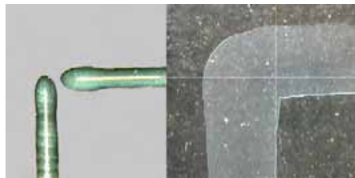
Figure 10- Overlapping Dots Form Continuous Lines
