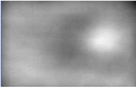
Fig.2-1 Panel map of Capacitance Measurement value (defect-free panel)
