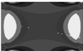
Fig. 13. Plot of an equivalent strain over the diffuser film at t = 90 sec.
