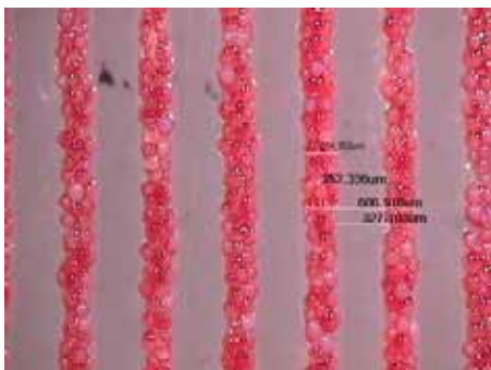
Figure 5. Optical micro-photograph of magenta/white microcapsule strips on ITO electrode.
