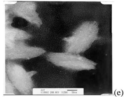
Figure 1. Microstructures of (a) MWNT (multi-wall nanotube) powders (b) dispersed CNT (c) MWNT/CuO nanocomposite powders (d) MWNT/Cu nanocomposite powders, and (e) MWNT/CuO nanocomposite powders (TEM).
