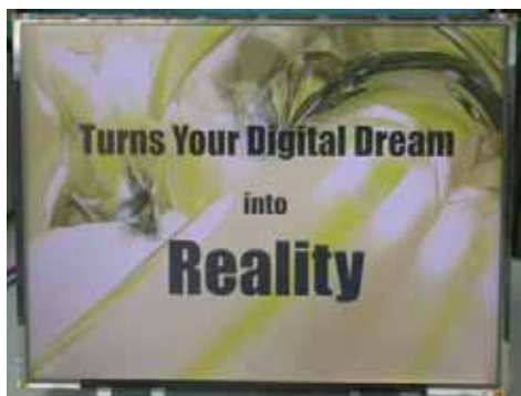
Figure 8. 14.1" TFT-LCD with integrated a-Si TFT gate driver using multi-thread driving
