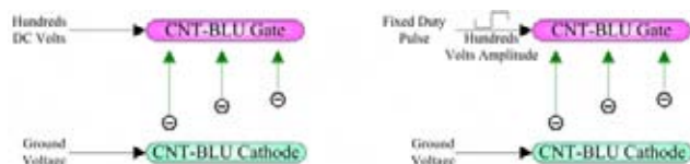
Fig. 2. Traditional driving methods for CNT-BLUs: DC driving method (left) and fixed pulse driving method (right).
