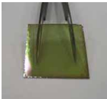
Figure 5. Image of the fully crystallized Si film on the mica substrate
